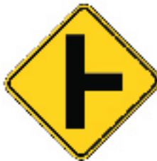
Side road enters highway ahead.
